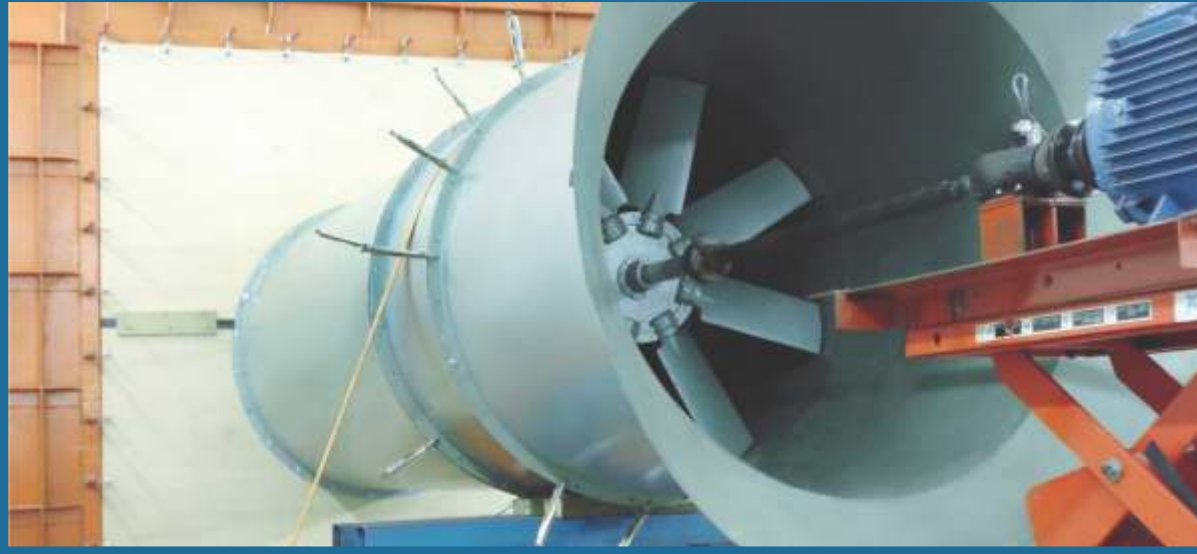
Testing of 'Ventech' Fan at AMCA accredited laboratory in Malaysia
